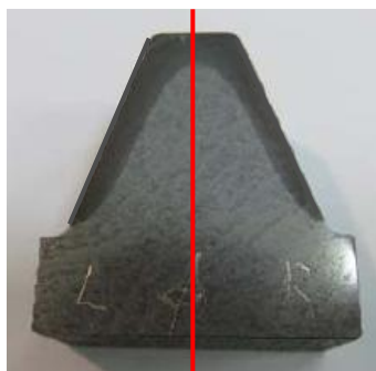
Qualified induction hardening and teeth grinding
